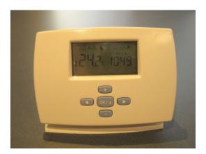
**TEI 6** (Radio Frequency Weekly Programmable Thermostat) – The TEI 6 Chrono-Thermostat enables the temperature to be regulated in one zone of the property at various times of the day. There is a 7 day program together with 9 standard or 4 user-defined programs. There is an LCD display for room temperature and time, a graphic display and a holiday mode option.
