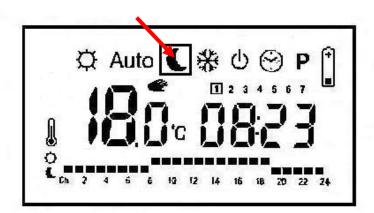
Move the controller into the "Moon" setting and reduce the temperature. The controller will not let the room temperature drop below this temperature when the radiator is off.
