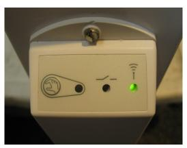
Push the button on the receiver for 5 seconds until the **green** light appears, indicating that the receiver is ready to be linked to the thermostat.
