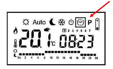
Move the controller into the "Clock/Time" setting, second from the right, using the left and right arrows.
