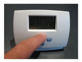
This can be tested this by pressing the plus (+) button the controls the temperature setting on the LCD display, to raise the temperature above the current room temperature. The LCD light will then flash across the button of the display.
