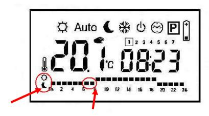
Each of the blocks along the bottom of the screen represent one hour. Move through the hours using the arrow keys and move them between the "Sun" and "Moon" setting by using the + and - keys.
