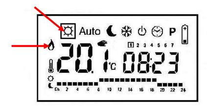
Put the controller into the "Sun" setting, use the plus and minus keys to choose the desired temperature. If the desired temperature is greater than the current room temperature, a flame will appear on the left hand side.
